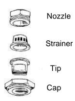
Figure 7.9 Parts of a nozzle
