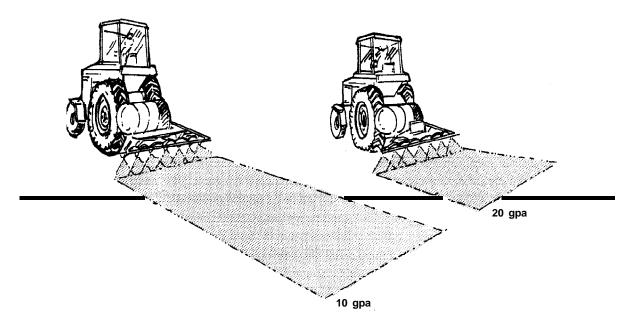
**Figure 6.1** Altering the volume applied by changing travel speed.
