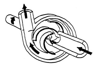
Figure 7.8 Centrifugal pump
