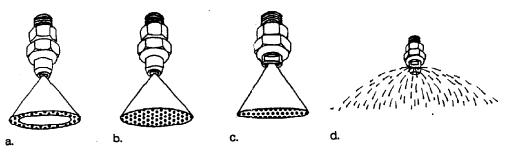
Figure 7.10 Nozzle types (a. hollow cone, b. solid cone, c. flat fan, d. flooding flat fan)
