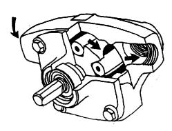
Figure 7.7 Roller impeller pump
