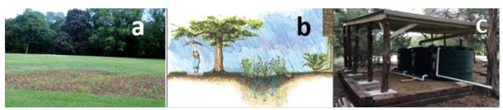
Figure 8: Rainwater harvesting options include passive collection through soil works and active collection in storage tanks. (a-rain garden, b-bioswale). (Photo a from NEXT.CC and b adopted from Natural Resources Conservation Service, and c-from Cypress Creek in Texas).
