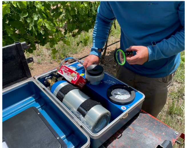
Quantifying water stress using a pressure "bomb" helps growers properly manage vine water requirements.
