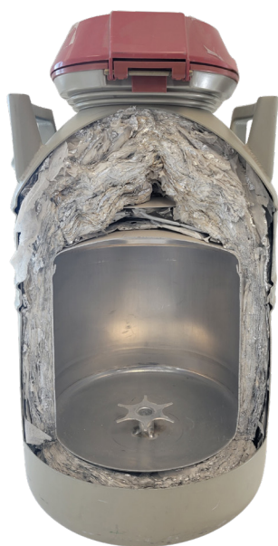
Figure 3. Split liquid nitrogen tank showing interior of the double chamber. Image credit: Katie H. Spanyers.
